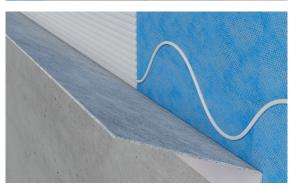
Now attach a sound insulation strip to the faces of the bathtub which later come into contact with the wall. Please make sure to leave at least 5 mm space to the upper edge for the silicone filling.
